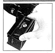
(4) After loading the batteries, insert the battery compartment cover into place, by coinciding protrusions at the upper end of the cover to notches on the body. Then revolve the fixing screw in the CLOSE direction (clockwise), with a coin, etc., while pressing the cover in place at the same time.
