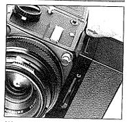
(2) Next, push the safety stop down while, at the same time, pulling the camera body away from the Motor Drive E with a slight lifting action.
