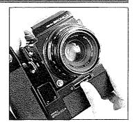
(6) When the camera body is inserted fully into place, the safety stop will spring up and lock the camera body. Please confirm that the safety stop is working at this time.
